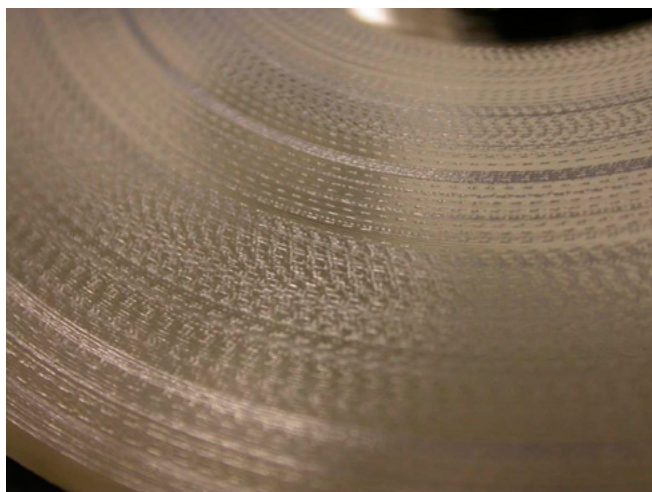
Figure 6. Here is a picture of a completely scratched and unrecoverable Hard Disk Drive Platter
